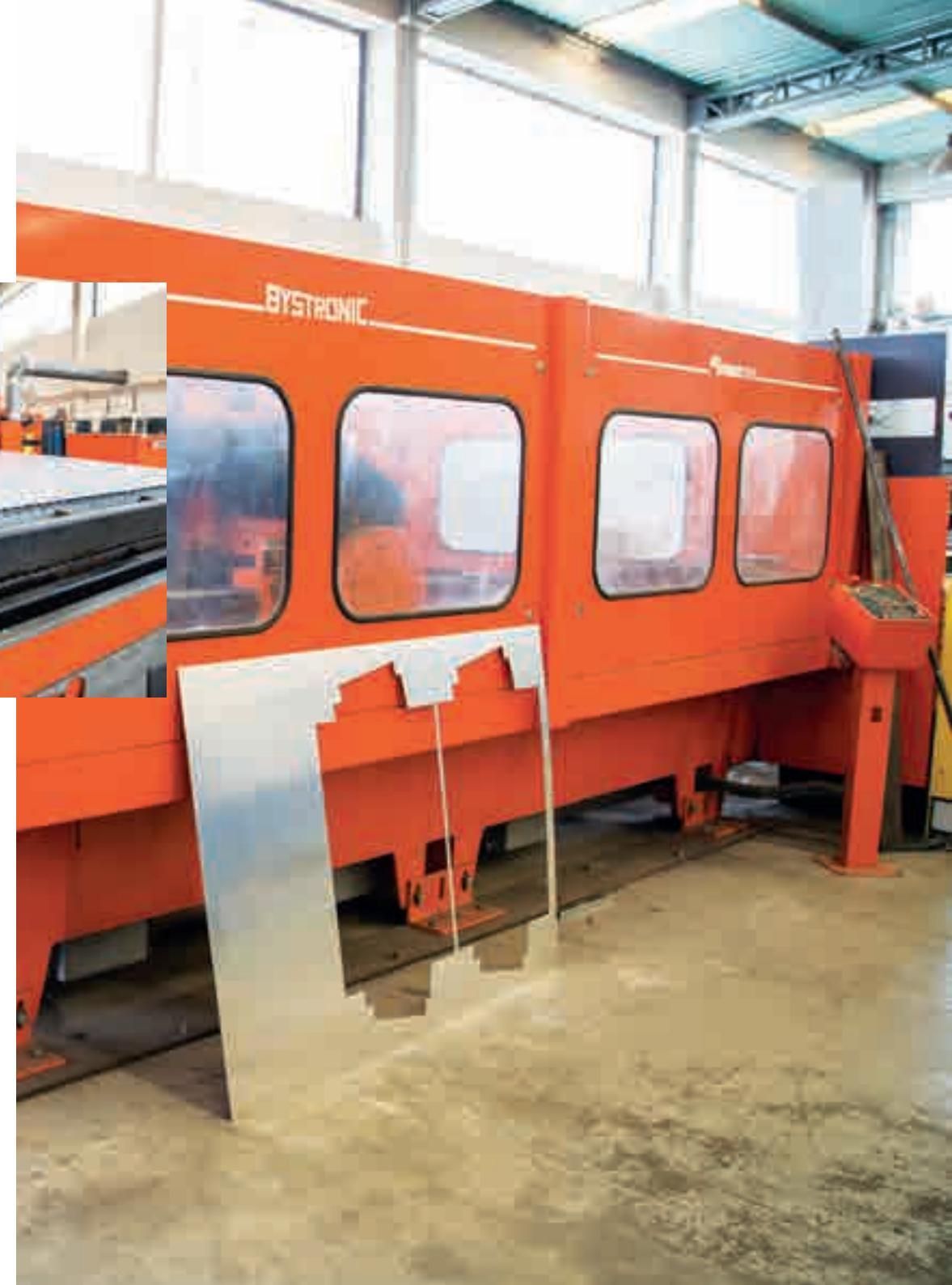
Metal sheet plates Laser cutting, stainless steel or aluminum. Thickness up to 8 mm in steel, 6 mm and 4 mm stainless steel, aluminum.
