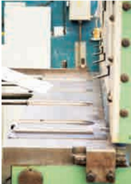
Metal sheet cutting by guillotine up to 10 mm thick.
