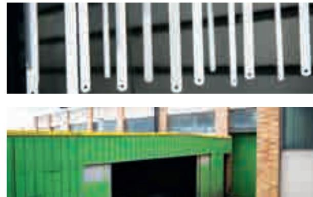
Electrostatic Painting system with static oven with 3,00x1,60x1,70 m. All pieces have pretreatment by degreasing and suitable to primary material to be used.
