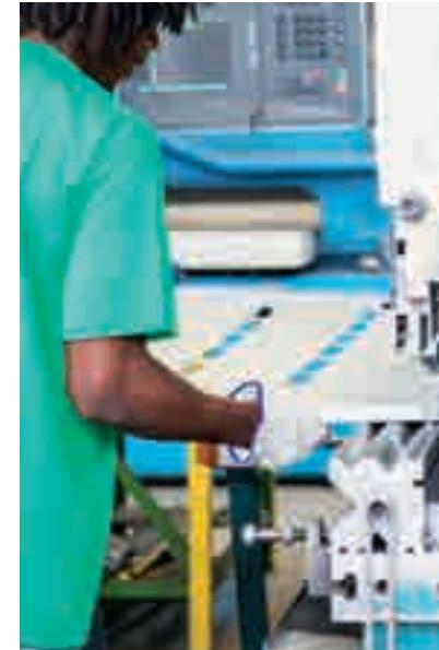
Bending of parts up to 3000 mm in length and 10 mm thickness. Different matrices and punches allow to get different angles and bending radius.
